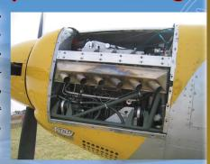
The Titan crew flew in with 3 of their Mustangs...one with a Rotax 912, one a Suzuki V-6, and the long awaited Honda 3.5L V-6, putting out an adequate 240 hp and cruising at around 3000 rpm. This engine coupled with the compact Neil Hintz gear drive (N.Z), and Whirlwind 4-blade constant speed 84" prop appears to be the package of choice from the factory...and it goes beautifully according to John Williams of Titan Aircraft and anyone else who has had the pleasure to see or feel it.
